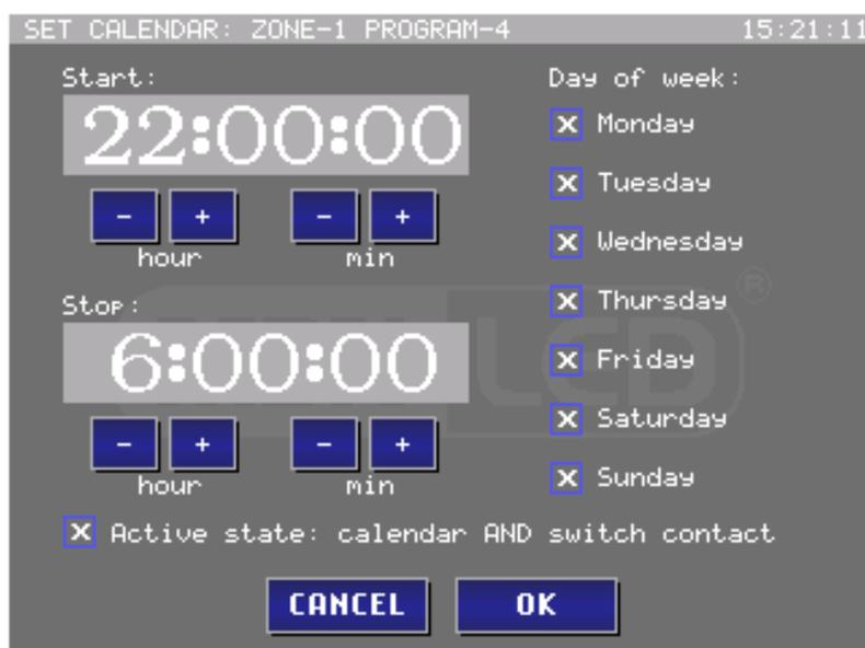
The calendar function can be connected with USM module contact feature. It means that the program is running only if the actual date and time between the calendar start-stop time and for the program selected contact sensor also active (closed).
