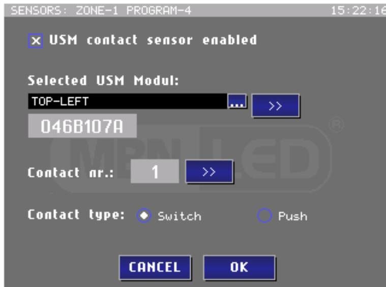
You can enter and edit a name for each USM module. This makes it easier to identify different devices.
